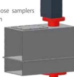
pipe protruding in the material flow that is provided with openings. Normally, these openings are turned in the direction of conveyance and close against a sealing gasket. At the time of sampling, the sample collecting pipe with its openings is turned against the direction of conveyance, so that sampling material can flow in. The sample material thus entered is discharged downwards through the air slide conveyor system by means of the sample collecting pipe.
